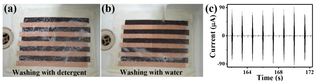
Figure 6. Washing process of the generator: (a) washing with detergent and (b) washing with water. (c) The output current of the generator after washing.
